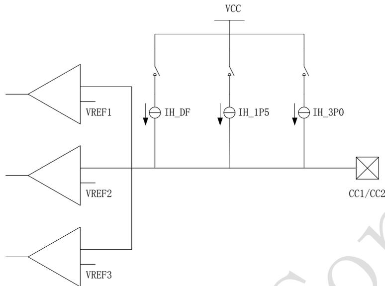
图 6. Plug and Orientation Detection Block
